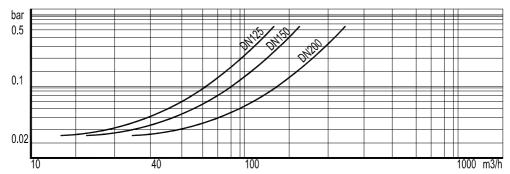
To determine the pressure drop of other mediums the equivalent water flow volume has to be calculated:  $V_W = \sqrt{\frac{Q}{1000}} \times V$
